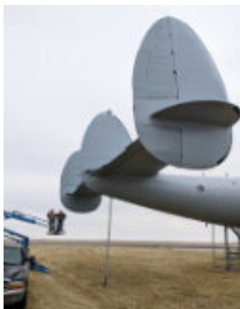
Mike Madden and Mike Welch install the last rudder (K. Drewelow photo)
